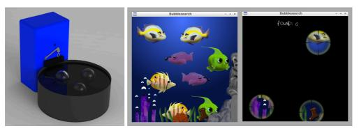
Figure 1. The Soap Bubble Interface with bubble generator and soap bubble basin. The basin has a diameter of approx. 50 cm. Generated bubbles drop onto the liquid surface where they float.
